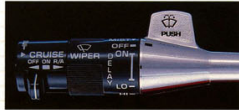
Electronic speed control and intermittent wiper shown on standard multi-function switch.
