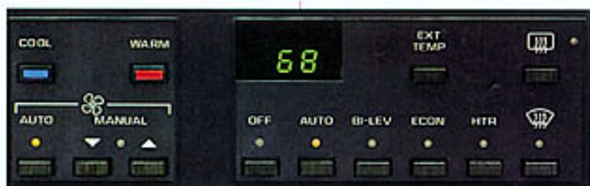
Electronic air conditioning lets you set desired temperature digitally.
