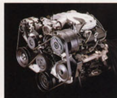
A 140-HP 3.1 Liter V6 with Multi-Port Fuel Injection is standard on Camaro RS Coupe. Features include high-energy ignition, electronic spark control and a single-belt accessory drive designed to never need adjustment.
