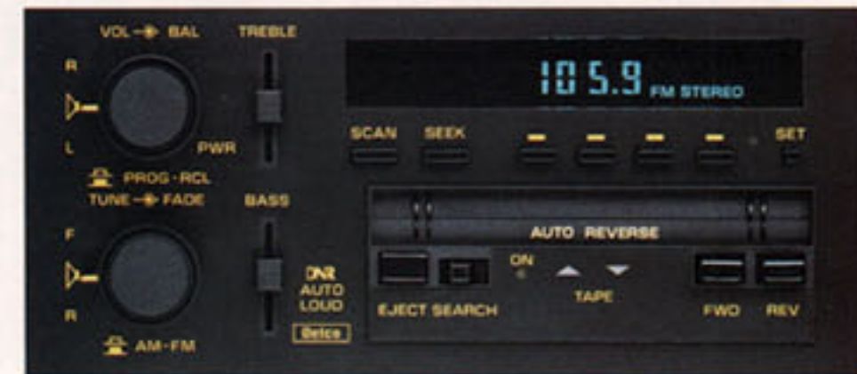
Electronically tuned AM/FM stereo with seek/scan, stereo cassette tape player with search and repeat, Extended Range Sound System and digital clock.
