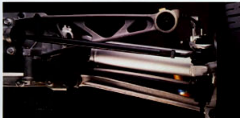
A sophisticated five-link independent rear suspension is standard on Corvette.
