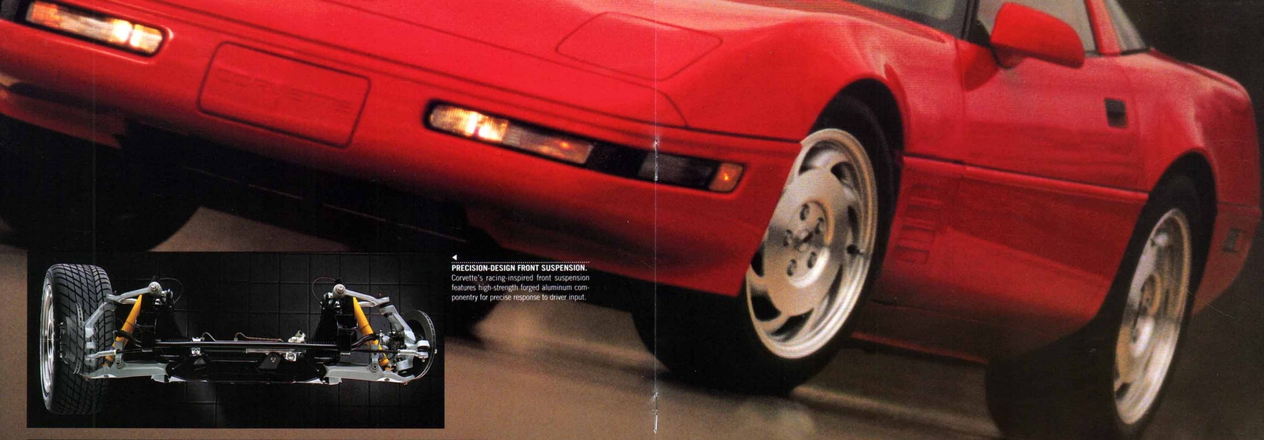
INDEPENDENT REAR SUSPENSION. A unique 5-link independent rear suspension with a transverse monoleaf spring helps put Corvette's power to the pavement.
