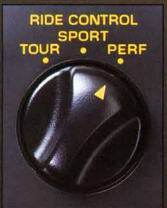
SELECTIVE RIDE & HANDLING PACKAGE. The optional Selective Ride and Handling Package allows the driver to select one of three suspension system settings via a console-mounted switch.
