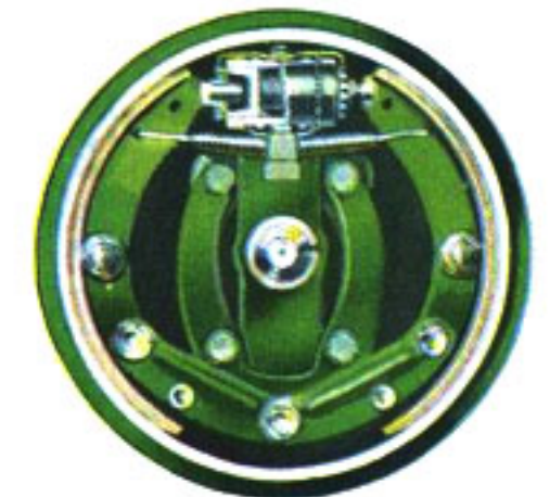
Double-articulated brake-shoe linkage promotes positive equalized braking and prolongs lining life.
