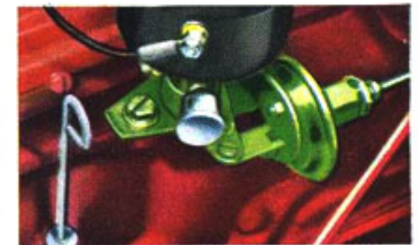
By means of the octane selector, the ignition timing may be set to get the most out of whatever grade of fuel is used.
