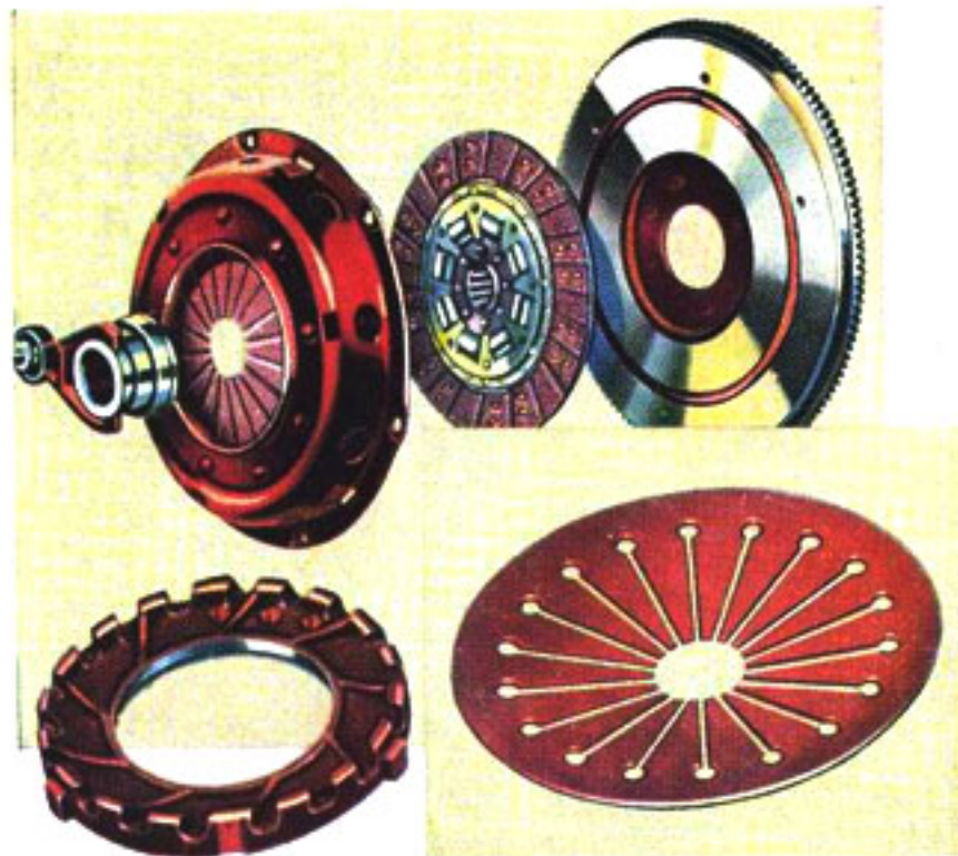
Low pedal-pressure and smooth engagement are features that distinguish the diaphragm-spring clutch. The 1940 clutch has improved disc cushioning.
