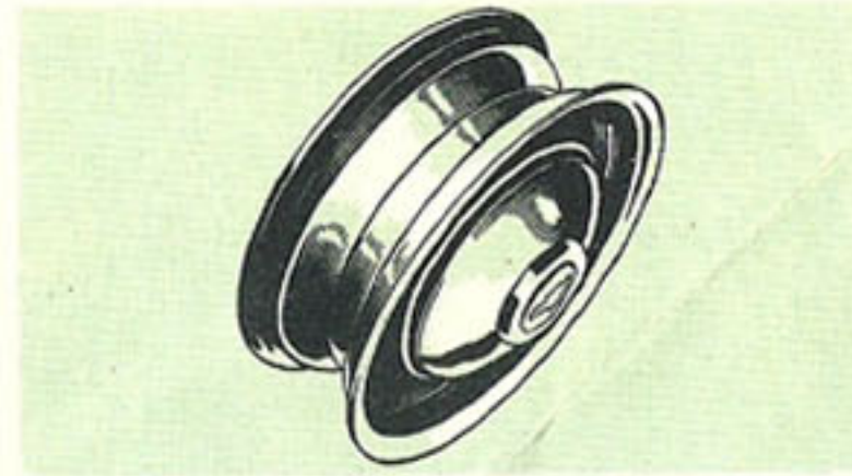
5-INCH WIDE BASE RIMS —widest in the low-price field—combine with low-pressure tires to make a large, soft riding "cushion".
