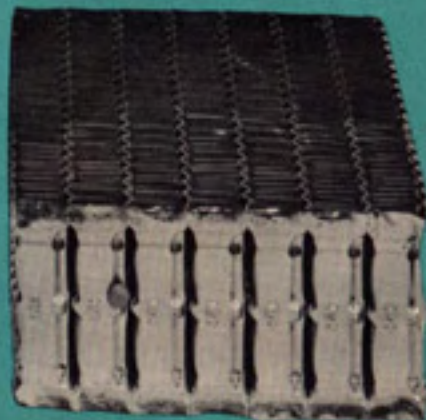
CROSS SECTION OF CELLULAR TYPE RADIATOR CORE
