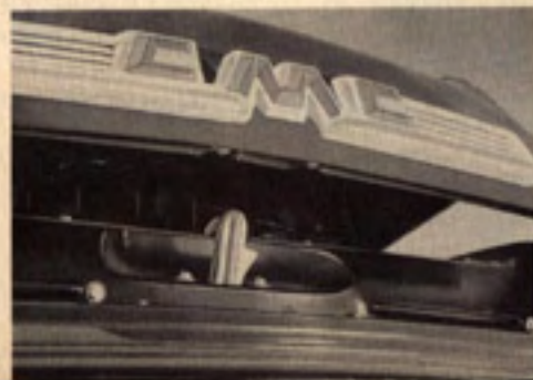
The new hood latch is positive in action, and easily accessible through the grille bars. A longer release lever is easy to get at and easy to operate.
