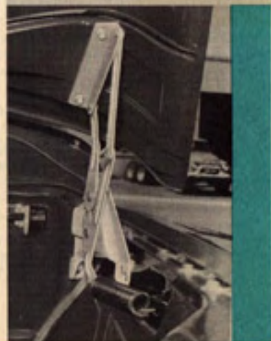
The new hood latch is positive in action, and easily accessible through the grille bars. A longer release lever is easy to get at and easy to operate.
