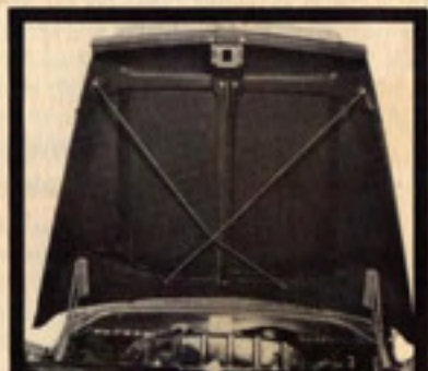
A new center hood reinforcement brace running the length of the hood ties the front and rear hood cross reinforcements for increased rigidity.
