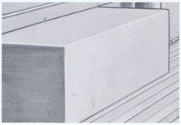
RECTANGULAR WHEELHOUSES permit efficient use of load space. They are standard in Chevrolet Step-Vans.
