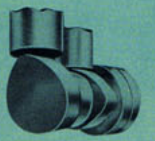
ECONOMY-CONTOURED CAMSHAFT cuts costs of delivery runs. Timing and lift of inlet and exhaust valves result in top fuel economy with high torque output in low and medium speed ranges. Saves gas in stop-and-go driving as well as when idling.
