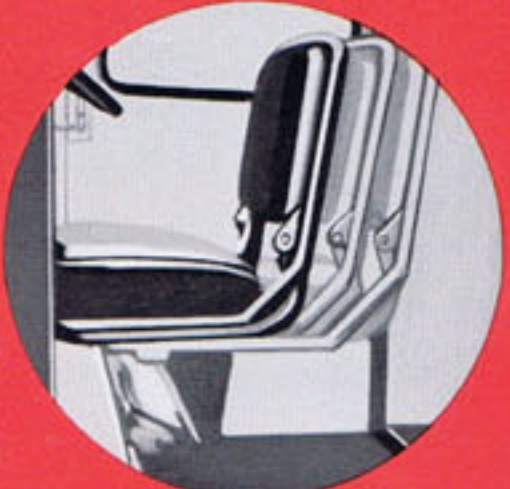
ADJUSTABLE SEAT moves forward or back, up or down. Folds under the steering wheel for easy access to the cargo area.
