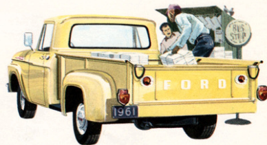
New Ford F-350 1-tonner with 132-in. wb., available with 9-ft. Styleside or Flareside box, Platform-Stake, Chassis-Cab, Chassis-Cowl or Chassis-Windshield. Max. GVW: 9,800 lb. (7,600 lb. for pickups). Flareside box (shown) has rolled edge flareboards, and running boards between cab and rear fender.
