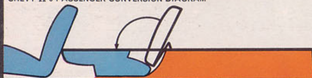
CHEVY II 6-PASSENGER CONVERSION DIAGRAM
