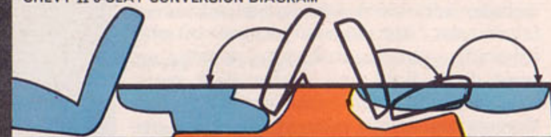
CHEVY II 3-SEAT CONVERSION DIAGRAM
