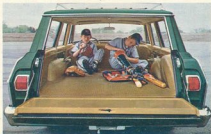
Nova Station Wagon Interior in saddle, offering 76 cubic feet of cargo space. Covered spare tire and wheel are conveniently carried upright in right rear quarter panel wall.
