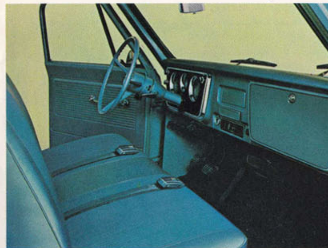
Standard cab interior: tough, washable vinyl over thick foam. Seatbelts, padded dash and sun visors are standard.
