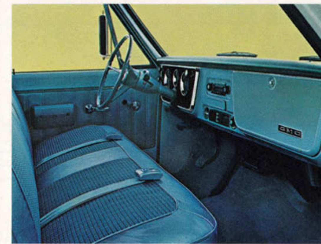
Custom cab interior: with deeply padded vinyl and cloth seats, dual armrests and bright metal trim on control knobs.
