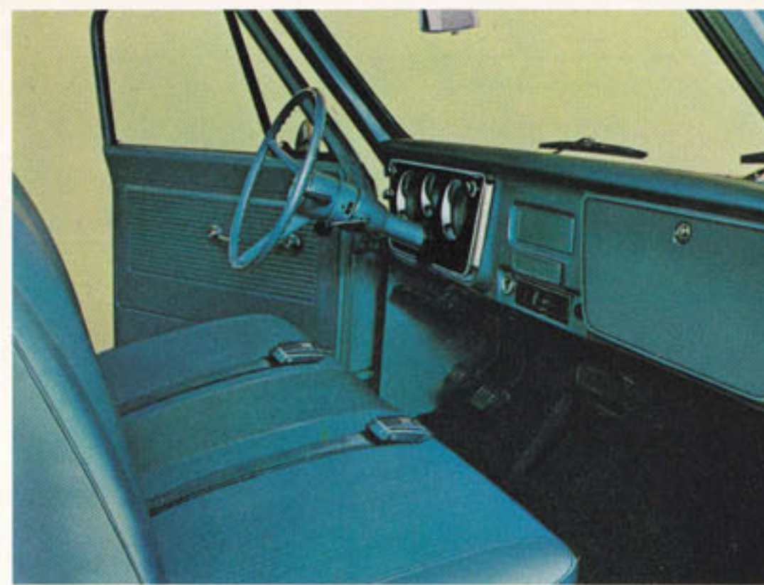
Standard cab interior: tough, washable vinyl over thick foam. Seatbelts, padded dash and sun visors are standard.
