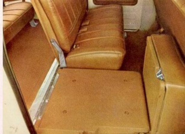
Cushion unclatches and folds forward. Backrest unclatches and folds down.
