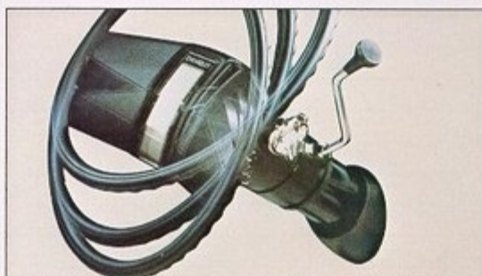
Comfortilt steering wheel. Flick a lever and swing the Comfortilt wheel up, down and in between. You can change to six different driving positions without ever leaving your seat. Available when automatic or 4-speed manual transmission is ordered.
