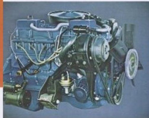
4.1 Litre (250 CID) In-Line Six gasoline engine
