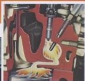
Electric glow plugs help provide efficient cold starting for the V8 diesel engine
