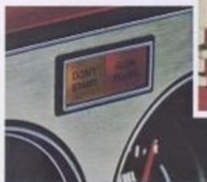
Instrument cluster includes alert lights for glow plugs and engine starting
