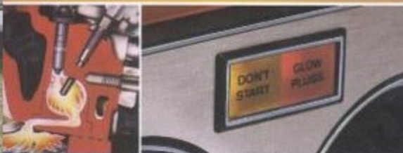
Glow plugs help provide instant, cold weather starting.
