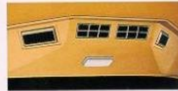
Suburban front and rear air conditioning*
