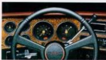
SLE instrument cluster with standard gauges and simulated woodgrain applique
