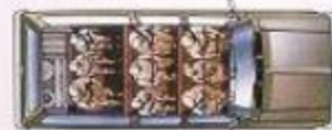
9-person seating with standard front bench seat and available folding center and removable rear bench seats
