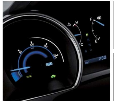
In addition to providing many standard gauges, such as the speedometer, Highlander Hybrid also features a hybrid system power meter that lets you know when the system is charging and shows electric power consumption.
