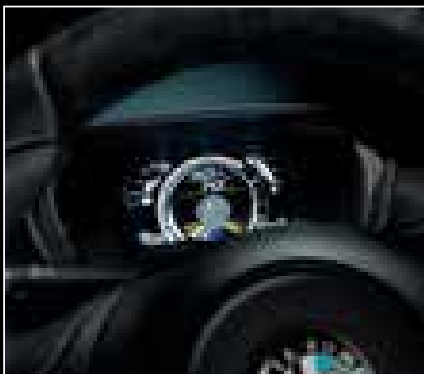
Full-digital instrument cluster with Thin Film Transistor (TFT) display and carbon fiber cluster surround
