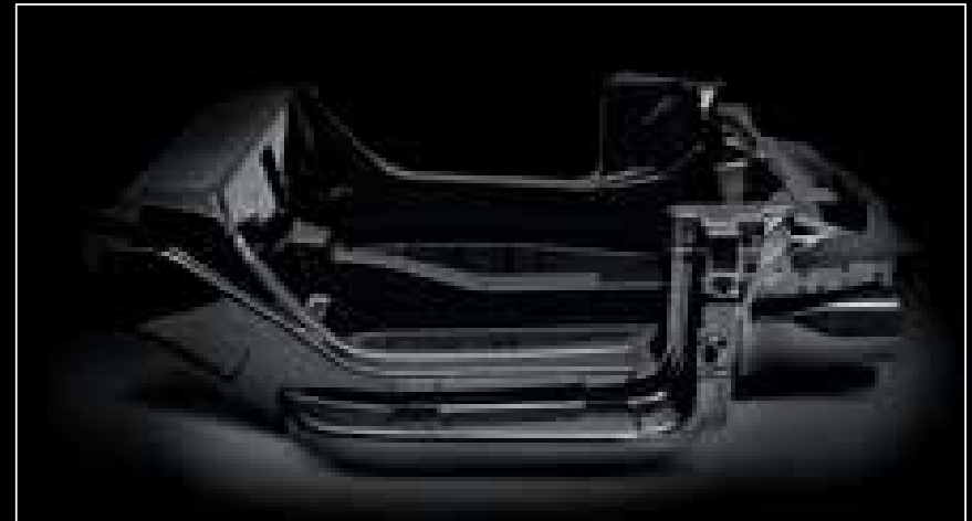
Genuine carbon fiber monocoque chassis
