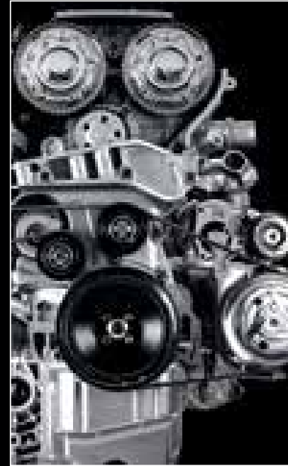
1750 turbocharged, aluminum, 4-cylinder engine
