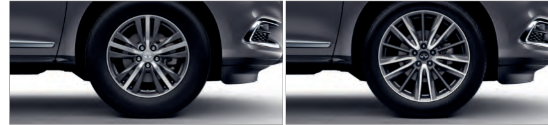
18 X 7.5-INCH TRIPLE 5-SPOKE ALUMINUM-ALLOY WHEELS
