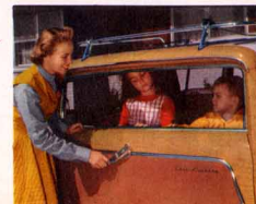
ROLL-DOWN REAR WINDOW disappears into tailgate at your command. The one-piece cargo door eliminates upper hinges—gives more loading room—improves ventilation.
