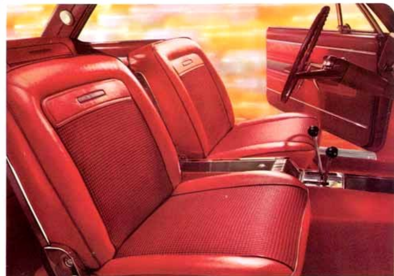
Twin-Stick Floor Shift permits five forward speeds. Optional on 440 and 440-H models.
