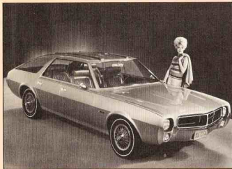
AMX III --An experimental fastback sports station wagon called the AMX III was exhibited first at the Chicago Auto Show in February, 1967. A novel feature which added versatility to the cargo area was the unique action of the tailgate which lifted up and, with scissor-action hinges, slid horizontally forward to rest on the roof. The model was finished in silver-gray.
