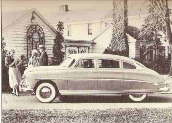
1953 HUDSON Wasp Sedan--This SuperWasp four-door sedan, built on a wheelbase of 119 inches, had a compression ratio of 7.2 to 1 with optional aluminum head and 6.7 to 1 with standard iron-alloy head. Hudson continued to emphasize "step-down" design and its lower center of gravity.
