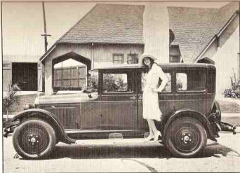
1927 NASH, Model 239--This four-door sedan in the Nash Special Six series was photographed in the fall of 1926 for national distribution to the press. Production at the Nash factories in Kenosha, Milwaukee and Racine for 1927 totaled 122,606 passenger cars. This model, built on a 113-inch wheelbase, weighed 3,170 lbs. and sold for $1,315. (Henry Austin Clark photograph.)
