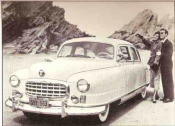
1949 NASH '600,' Model 4978 --To its completely redesigned 1949 line Nash Motors gave the name "Airflyte." New features included one-piece curved windshield, all wheels enclosed and the "uniscop" cluster of instruments.
