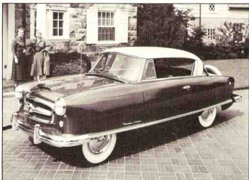
1953 NASH Rambler, Model 5327--This is the Rambler Country Club hardtop for 1953. Note the "N" on the gas cap. All Rambler models were built that year on a 100-inch wheelbase.
