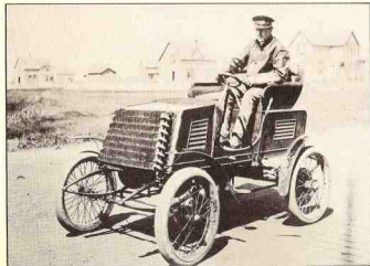
1901 RAMBLER, Model A--This model, designed by Charles T. Jeffery (at the wheel), was the first car built in the Kenosha plant, acquired by Jeffery in 1900 from the Sterling Bicycle Company. Note the engine is located in front, with the vehicle steered by a wheel located on the left side.
