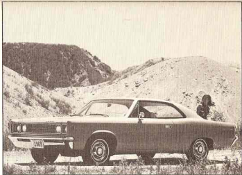
1969 REBEL, Model 6919--Wheelbase and overall length of the Rebel remained at 114 inches and 197 inches, respectively, with the station wagon's overall length at 198 inches. The new grille is highlighted in this photograph of the hardtop in the basic Rebel series.
