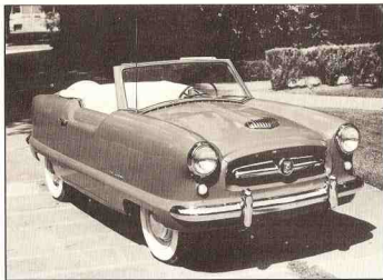
1954 METROPOLITAN, Model 541--In March, 1954, Nash introduced a completely new small car, built in England by Austin and Fisher-Ludlow, to Nash specifications. With an 85-inch wheelbase, it had a 42-h.p. engine which offered up to 40 miles per gallon. A two-door hardtop also was offered.
