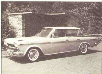
1960 RAMBLER Ambassador, Model 6089-2--A "compound wrap-around" windshield was introduced on Ambassador models in 1960. A Rambler American with automatic transmission won the annual Mobilgas Economy Run, achieving 28.35 mpg.
