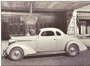
1937 NASH, Model 3782--The 1937 Ambassador coupe, with spare tire mounted in the rear deck, had two extra seats that swung out from the rear of the body to provide room for two extra passengers, making the coupe a five-passenger model. Wheelbase was 125 inches. Price: $855.
