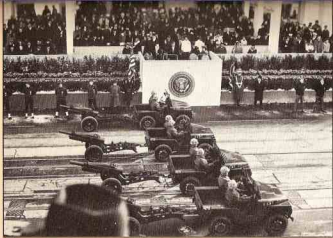
MIGHTY MITES --Standing at attention during his inauguration as President was John F. Kennedy as four Mighty Mite four-wheel-drive, air-borne vehicles built by American Motors passed by. From January, 1960 to January, 1963, a total of 3,922 Mighty Mites, powered by aluminum V-4 engines designed by American Motors engineers, were built in Detroit for the U.S. Marine Corps.
