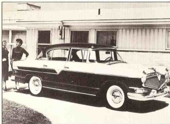
1956 HUDSON Wasp, Model 35645-2--This Wasp sedan was powered by the L-head engine that had been used in the Hudson Jet prior to the merger. In 1956, a total of 22,588 Hudsons were produced at Kenosha.
