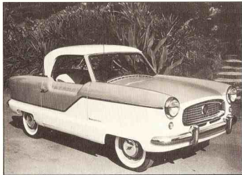
1956 METROPOLITAN, Model 562--On April 9, 1956, American Motors announced its new British-built Metropolitan, available in both soft-top and hardtop convertible models. New features included a 52-h.p. Austin engine, up 24% over previous models.
