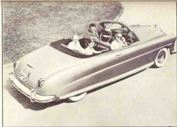
1948 HUDSON Convertible Brougham--Hudson models in 1948 had the lowest center of gravity of any U.S.-built cars. Drive-Master automatic transmission was optional in the Super Six, Commodore Six and Eight series.
