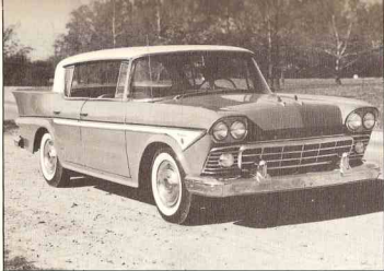
1958 RAMBLER Rebel, Model 5829-2--Rambler also offered a V-8 engine on 108-inch-wheelbase models; horsepower was 215 on this Rebel hardtop sedan. Beginning with 1958 models, Rambler pioneered a new "deep-dip" rust-proofing system, dipping all bodies in a 15,000-gallon tank of special primer.
