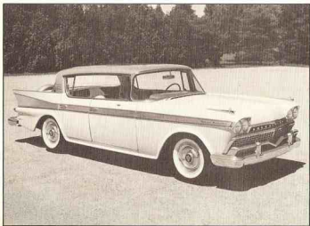
1958 RAMBLER Ambassador, 4-Door Hardtop, Model 5889-2--Beginning with the 1958 model year, American Motors dropped the Nash and Hudson trade names to concentrate completely on Rambler. The "senior" series was the Rambler Ambassador, built on a 117-inch wheelbase and powered by a 270-h.p. V-8 engine.
