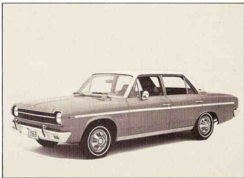
1969 RAMBLER 440, Model 6905-5--All American Motors cars in 1969 included head restraints as standard equipment, a cable-controlled accelerator system with a suspended pedal, a new smaller, lighter battery with translucent case and new Guard-Glo safety headlamps, featuring stand-by filaments.
