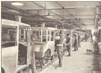
1921 ESSEX bodies on the Detroit assembly line were manufactured, to a large extent, of wood, as this picture illustrates. Because of the first postwar depression, Hudson-Essex sales in 1921 fell off to 27,143.
