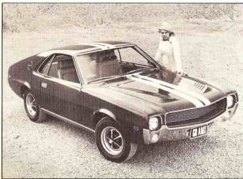
1968 AMX, Model 6839-7--Widespread interest among performance-minded enthusiasts was generated by the sporty two-seater AMX, introduced in mid-February. It featured four-barrel V-8 power and such performance items as rear traction bars, large-diameter front sway bar, heavy-duty springs and shocks and wide profile fiberglass belted tires.
