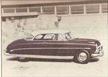
1952 HUDSON Wasp Hardtop--In 1952 Hudson introduced the low-priced Wasp series, built on a 119-inch wheelbase and powered by the H-127 six-cylinder engine. Styling that year was known as "Hudson-Aire Styling."
