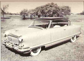
1953 NASH Ambassador, Model 5377--Shown is the Country Club hardtop in the Ambassador series for 1953. Power steering was offered for the first time as optional equipment, as was the LeMans Dual Jetfire engine.
