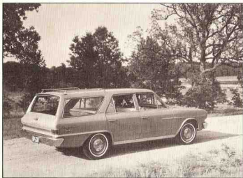
1964 RAMBLER American 330, Model 6408-2--Popular station wagon models also got a complete new look in 1964. The wider tailgate featured a roll-down rear window, and cargo capacity was boosted nearly 20 per cent. Fourteen-inch tires were standard, with 15-inch tires optional, on all Americans.
