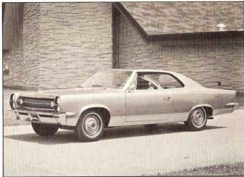
1967 AMBASSADOR DPL, Model 6789-7--Wheelbase of the 1967 Ambassador was increased from 116 to 118 inches, and overall length from 200 to 202.5 inches. Width also moved up 3.9 inches. Calendar year production of AM cars: 229,058.
