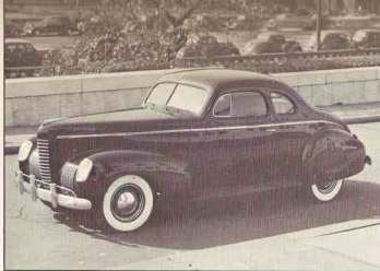
1939 NASH, Model 3925--This Ambassador Six coupe, seating three passengers, was built on a wheelbase of 121 inches. Eight-cylinder models were mounted on a 125-inch wheelbase. F.o.b. price of this car was $925.
