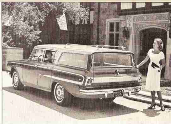
1962 RAMBLER Ambassador V-8, Model 6286-5--The Ambassador series, Rambler's luxury compact, was nine inches shorter than 1961 models, built on a 108-inch wheelbase. No dimensional changes were made in the interior, and the 250-h. p. V-8 engine was standard, with a 270-h. p. version optional.
