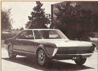
AMX II --A modified version of the original AMX was the AMX II, which featured a "Y" rear window to blend with rear deck contours, and overall length of 187 inches. Safety tail lights with green, amber and red lenses would give cars behind immediate indication of the driver's intentions or actions.
