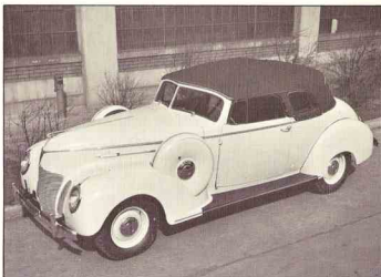
1939 HUDSON Convertible Brougham--This model introduced a new Country Club series available with both six and eight-cylinder engines giving respectively 101 and 122 horsepower, mounted on 122-inch wheelbase. Two sedan models were available on a 129-inch wheelbase.
