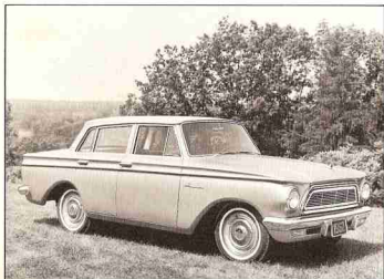
1962 RAMBLER American, Model 6205-5--Styling stability continued to keynote the Rambler American as the only significant appearance change in 1962 was the redesigned grille. A new optional automatic-clutch transmission called "E-Stick" was offered in the American series. The cost was only $59.50.
