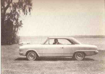
1964 RAMBLER American 440-H, Model 6409-7--One of the top American models for 1964 was this smart hardtop. Glass area on all Americans was increased 37 per cent, to provide improved eye-level visibility. Curved glass side windows, a seven-fold increase in galvanized metal for greater rust resistance and 33,000-mile or 3-year chassis lubrication intervals were featured.
