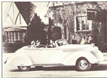
1937 HUDSON Convertible Brougham--This eight-cylinder model was one of the most popular offered in 1937. Optional equipment that year included the new Selective Automatic Shift: "Gear selection is made with the Electric Hand, and with a lift of the toe at any speed, gears shift automatically."
