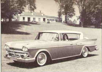
1959 RAMBLER Ambassador, Model 5989-2--The Ambassador series incorporated the luxury, comfort and performance of larger U.S. cars, yet retaining compactness. The Ambassador had a grille different in design from the 108-inch wheelbase models. The eight-cylinder engine developed 270 horsepower.
