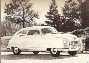
1950 NASH Ambassador, Model 5069--The most noticeable appearance change in Nash cars for 1950 was a larger curved rear window. Ambassador models took top honours in many stock-car events throughout the United States and Europe in 1950. Horsepower of the overhead-valve engine was 115.
