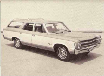
1968 AMBASSADOR DPL, Model 6888-5--Seven models were offered in the 1968 Ambassador series, including this DPL station wagon. The new V-profile air-foil-type grille was of injection-molded ABS plastic. Handling packages offered included front sway bar and heavy-duty springs and shocks.
