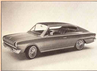
1964 RAMBLER Tarpon --First shown at the national convention in Detroit of the Society of Automotive Engineers in January, 1964 was this experimental fast-back model called the Rambler Tarpon. The car, which was not put into production, had a wheelbase of 106 inches, overall length of 180 inches and width of 52-1/2 inches. The model was finished in gold-flecked vermillion.
