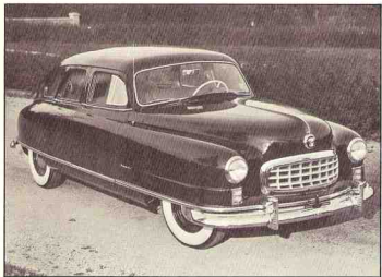
1949 NASH Ambassador, Model 4978 --All Nash cars in 1949, including the Ambassador, featured single-unit construction. The new models stood 62 inches high, six inches lower than 1948 models. Production totaled 142,592, a record. Twin convertible beds were offered for the first time.
