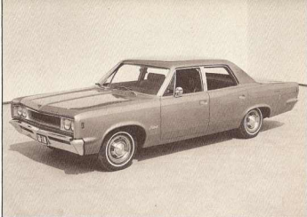
1968 REBEL 770, Model 6815-5--All 1968 American Motors cars except Rambler Americans featured new flush-mounted rectangular outside door handles and a pre-set door locking system.
