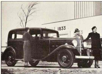
1933 NASH Big Six, Model 1127--Photographed at Chicago's Century of Progress fair in 1933 was this Nash town sedan which had an f.o.b. price of $695. In that year Nash located the light dimmer switch on the floor between the brake and clutch pedal. This model had a wheelbase of 116 inches.
