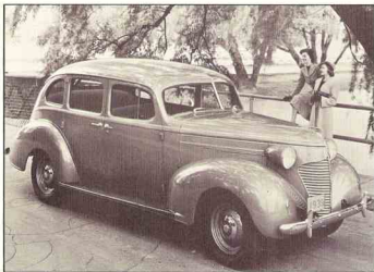
1939 HUDSON 112 Touring Sedan--This low-priced six-passenger sedan, mounted on a wheelbase of 112 inches, had an 86-horsepower engine. The hood ornament was plastic and had a light inside. Hudson emphasized its "Handy Shift," a shift lever mounted on the steering column.
