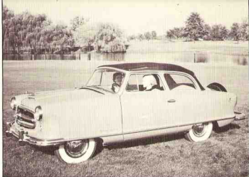
1953 NASH Rambler, Model 5321--Farina's styling was applied to all Rambler models in 1953. The continental rear tire mount was standard equipment on all convertibles and hardtops in the Rambler series.
