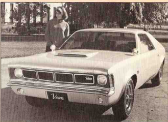
VIXEN --A landau-type roof with canted vents in the rear characterized the Vixen. The vents were angled at 45 degrees to increase visibility when the car was parked or when the driver backed up, and a sliding quarter window permitted flow-through ventilation when desired.
