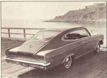
1965 RAMBLER Marlin, Model 6559-7--On February 10, 1965, American Motors announced details of its all-new six-passenger fastback hardtop which it called the Marlin. Dimensions included 112-inch wheelbase, 195-inch overall length, 54-inch height. Power-disc brakes were standard. In the 1965 model year, a total of 10,327 Marlins were produced.
