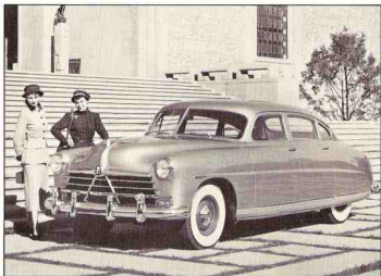
1950 HUDSON Pacemaker Sedan --Hudson in 1950 continued to emphasize its unique "Step-Down" design and Monobilt construction. This low-priced Pacemaker sedan was only 201.5 inches in overall length and was built on a 119-inch wheelbase. Horsepower of the six-cylinder engine was 112.
