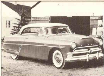
1954 HUDSON Wasp Hardtop--Extensive styling changes highlighted 1954 Hudson models, including a one-piece curved windshield and new front end. Shown is the Hollywood hardtop model in the Wasp series.
