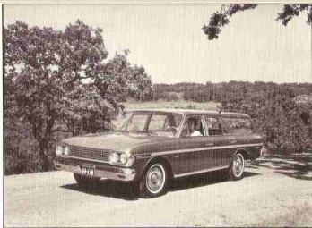
1964 RAMBLER Classic 770, Model 6418-5--A 198-horsepower V-8 engine was optional on all Classic models in 1964. The standard six-cylinder engine developed 127-horsepower, with a 139-horsepower option available. New on Classic and Ambassador models was the Adjust-O-Tilt steering wheel.
