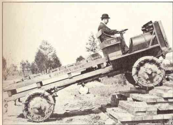
1915 JEFFERY TRUCK--The versatility of the Jeffery Quad truck was dramatically demonstrated by this derby-topped engineer. Thousands of these vehicles were purchased by the French and British governments for use in World War I. The Quad was advertised: "Drives, brakes and steers on all four wheels."
