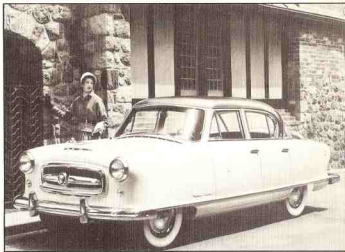
1954 NASH Rambler, Model 5425--In 1954, Nash introduced a completely new Rambler model, this four-door sedan, built on a 108-inch wheelbase. In that year, Nash became the first manufacturer to offer a complete air-conditioning system with the entire unit located under the hood.
