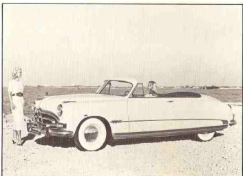
1951 HUDSON Hornet Convertible--The "fabulous Hornet" was introduced by Hudson in 1951. In addition to a convertible, the series included a four-door sedan and a club coupe. Powered by a new high-compression H-145 six-cylinder engine, the Hornet also offered four-speed Hydra-Matic Drive.
