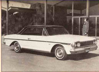
1964 RAMBLER Typhoon --To introduce its all-new 232-cubic-inch "Torque Command" six-cylinder engine in the spring of 1964, American Motors offered the new engine in a limited number of Rambler Typhoon two-door hardtops. All 2,520 built were finished in Solar yellow with a black roof and black side spear and grille accents.
