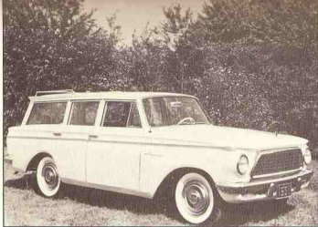
1961 RAMBLER American, Model 6108-2--With the popularity of the American series continuing to mount, American Motors added a four-door station wagon and a convertible to the line in 1961. A 125-h.p. overhead-valve six-cylinder engine was standard on all Customs and optional equipment on Super and Deluxe models in the American series.
