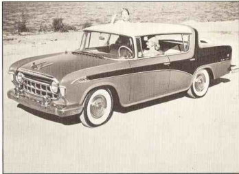
1956 RAMBLER, Model 5615-2--An all-new Rambler series, with the latest in compact styling and engineering, was introduced in 1956. All models featured a new 120-h.p. overhead-valve engine and were built on a wheelbase of 108 inches. A new body style was this four-door hardtop sedan.
