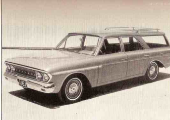
1963 RAMBLER Classic 660, Model 6310-2--Both Classic and Ambassador station wagons were available in two-seat or three-seat versions, the latter with side-hinged tail-gate doors. All 1963 Classic and Ambassador wagons featured hidden storage compartments in the rear cargo floor. On March 1, 1963 a new 198-hp V-8 engine was introduced as an option on all Classic models.
