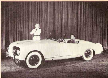
1952 NASH-HEALEY, Model 25262 --First shown at the Chicago Automobile Show in February, 1952, this Nash-Healey sports roadster was styled by Pinin Farina. The chassis was built by the Donald Healey Co. of Warwick, England; engine and transmission were built by Nash in the U.S., and the body by Farina in Italy.
