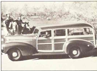
1941 HUDSON Station Wagon--This model, available with either a six or eight-cylinder engine, was mounted on a 121-inch wheelbase. With factory shipments of 79,529 cars, Hudson Motor Car Co. realized a $3,756,418 profit in 1941.
