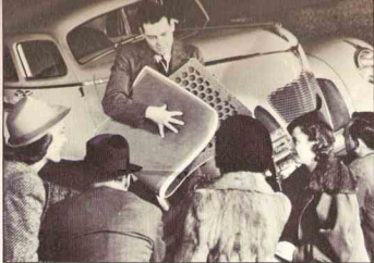
1939 HUDSON Sedan--Foam rubber cushions, later available on all U.S. makes, were introduced by Hudson in 1939, along with the dash-locking safety hood and vertical mounting of the spare tire in the trunk compartment.
