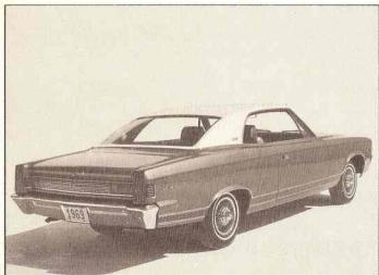
1969 AMBASSADOR SST, Model 6989-7--The most pronounced changes in American Motors' 1969 line were in the Ambassador series. The wheelbase was increased to 122 inches, and overall length went up to 206.5 inches for sedans and hardtops and 207 inches for station wagons.
