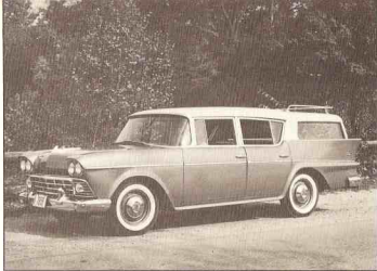
1958 RAMBLER Six, Model 5818-1--New rear fenders, dual headlights, step-on parking brake and new grille were among more than 100 improvements made on 1958 Rambler models. Pictured is the 127-h.p. six-cylinder Super Cross Country station wagon model, the top seller that year.
