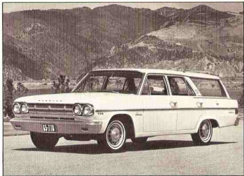
1965 RAMBLER Classic 770, Model 6518-5--Torque Command six-cylinder engines were basic powerplants for all 1965 Classic models, with the 198-HP 287-cubic-inch V-8 offered again as an option, plus the addition of a 270-HP 327 V-8. "Lustre-Gard" acrylic enamel paint finish was a new feature on all cars.
