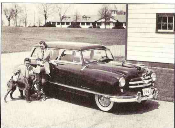
1951 NASH Rambler, Model 5124--Shown here is the 1951 Custom two-door station wagon, powered by a six-cylinder 82-horsepower L-head engine. Weight of this five-passenger model was only 2,515 lbs. Nash production also was hampered by effects of the steel shortage.
