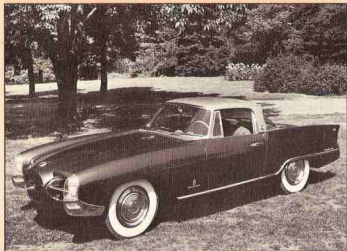
RAMBLER Palm Beach --This sport model, powered by a 90-h.p. Rambler six-cylinder engine, was designed and built in early 1956 by Pinin Farina in Italy. Exhibited at automobile shows in the United States and Europe, it was not put into production. Wheelbase was 101.5 inches.
