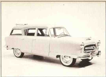
1954 NASH Rambler, Model 5428--Another new Rambler model that bowed in 1954 was this four-door station wagon, also on a 108-inch wheelbase. Known as the "Cross Country," it featured a "dip" in the roof that was to become a Rambler trademark, and a roof rack as standard equipment. Production of Nash cars dropped sharply to 67,192 in 1954.
