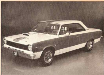
1969 SC/RAMBLER HURST --Production of this special high-performance Rambler Rogue was limited to 500 units and was quickly oversubscribed. The cars were modified by Hurst Performance, Inc., of Detroit, and were equipped with 390-cubic-inch V-8 engines and all performance options were standard.
