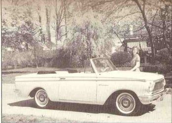
1961 RAMBLER American, Model 6107-2--The new Rambler American convertible, introduced in early 1961, was the lowest-priced U.S.-built convertible and the only such body type with single-unit construction. The completely restyled American series was more compact than ever-- 5.2 inches shorter and 3 inches narrower than 1960 models.
