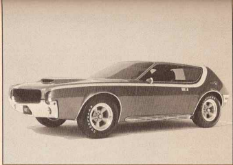
AMX-GT --This prototype of a two-passenger, high-performance GT (Grand Touring) super sports car was shown first at the International Auto Show in New York in April, 1968. The fiberglass body was mounted on a 37-inch wheelbase.
