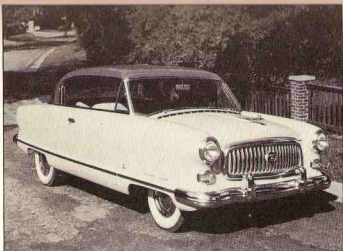
1953 NASH Statesman, Model 5357--Here is the Statesman custom hardtop for 1953. Nash advertising emphasized strength and safety of its unitized or "Air-flyte" construction.
