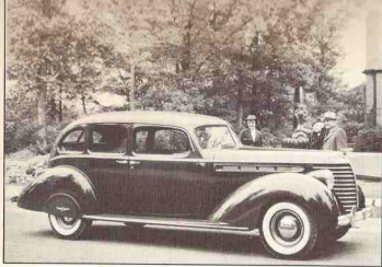
1938 HUDSON Touring Sedan--Designated as Model 87, this eight-cylinder Hudson was available on a wheelbase of 122 or 129 inches. Horsepower was increased to 122. Hudson shipped 51,078 cars in 1938.
