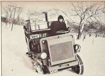
1914 JEFFERY TRUCK--Poor roads, covered with snow and ice, posed few problems to this 1914 Jeffery Quad truck. With power applied to all four wheels, it could manage any terrain. The only problem was keeping the driver warm.
