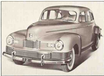
1946 NASH Ambassador, Model 4660--In resuming production, Nash in 1946 built only six-cylinder engines. This Ambassador four-door sedan had a 112-horsepower powerplant. Nash opened a 204-acre proving ground near Burlington, Wisconsin that year.
