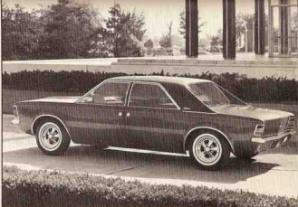
CAVALIER --The Cavalier, which had an overall length of 175 inches, introduced the possibility of interchangeability of body panels. Right front fender and left rear fender were identical, as were their opposite quarter panels. Hood and deck lid were the same, as were front and rear bumpers.
