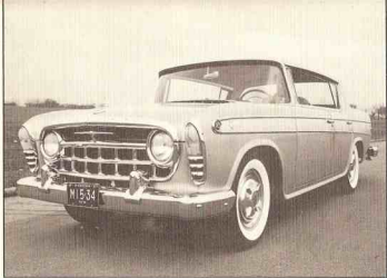
1957 RAMBLER Rebel, Model 5739-2--In 1957, Rambler brought out this limited-edition model of high performance. About 1,500 Rebels, all painted silver with gold-anodized spears, were built. The 108-inch-wheelbase car was powered by American Motors' new 255-h.p. V-8 of 327 cubic-inch displacement.
