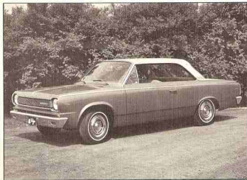
1966 RAMBLER American Roguo, Model 6609-7--New to the Rambler American series for 1966 was the two-door Roguo hardtop featuring a unique two-tone finish in which roof and rear deck were painted the same color. All American models were three inches longer forward of the windshield but, at 181 inches overall length, continued to be the shortest cars built in the United States.
