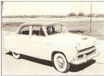
1953 HUDSON Jet--Hudson's long-awaited "light" car, the Jet, made its appearance early in 1953. Available with standard transmission, overdrive or Hydra-Matic, the completely new series was built on a 105-inch wheelbase. Horsepower of the six-cylinder economy engine was 104. Body by Murray.
