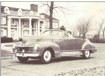
1946 HUDSON Super-Six Convertible--The principal appearance change from 1942 models was a completely new front end for 1946. All Hudson models that year were built on a wheelbase of 121 inches.
