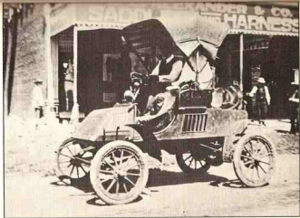
1903 RAMBLER, Model F--This car and the model shown to the left sported steering wheels which the owners installed, replacing tiller steering. It was in 1903 that Thomas S. Jeffery announced he would not pay the royalties on the Selden automobile patents. Production for the year totaled 1,350.
