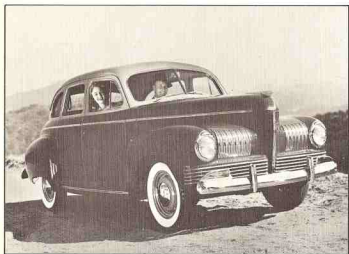
1941 NASH '600,' Model 4140--The publicity announcement of the revolutionary new Nash '600' stated prophetically: "In automotive history, the year 1941 will probably be noted principally for the introduction of a new kind of automobile body construction." With this new line, Nash pioneered single-unit construction, or, as it was called then "unitized" construction.
