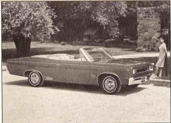
1967 RAMBLER Rebel SST, Model 6717-7--The Classic became the Rebel beginning with the 1967 model year. Overall length was increased to 197 inches (station wagons, 198 inches). The SST distinguished the top-of-the-line models.
