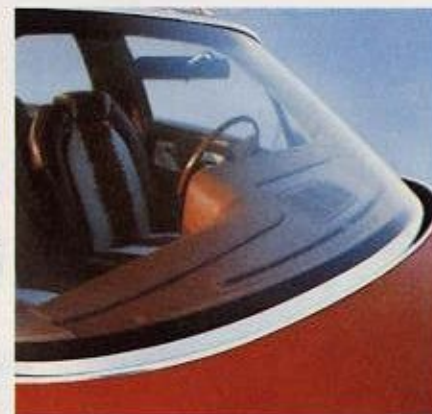
Electric windshield wipers are completely hidden when not in use—nothing interferes with Pacer's remarkable forward visibility. Unique "wet-arm" washers assure a clean sweep.
