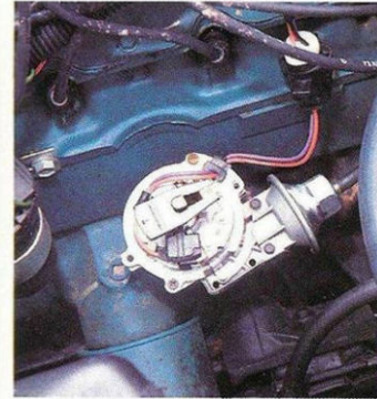
Electronic ignition system
