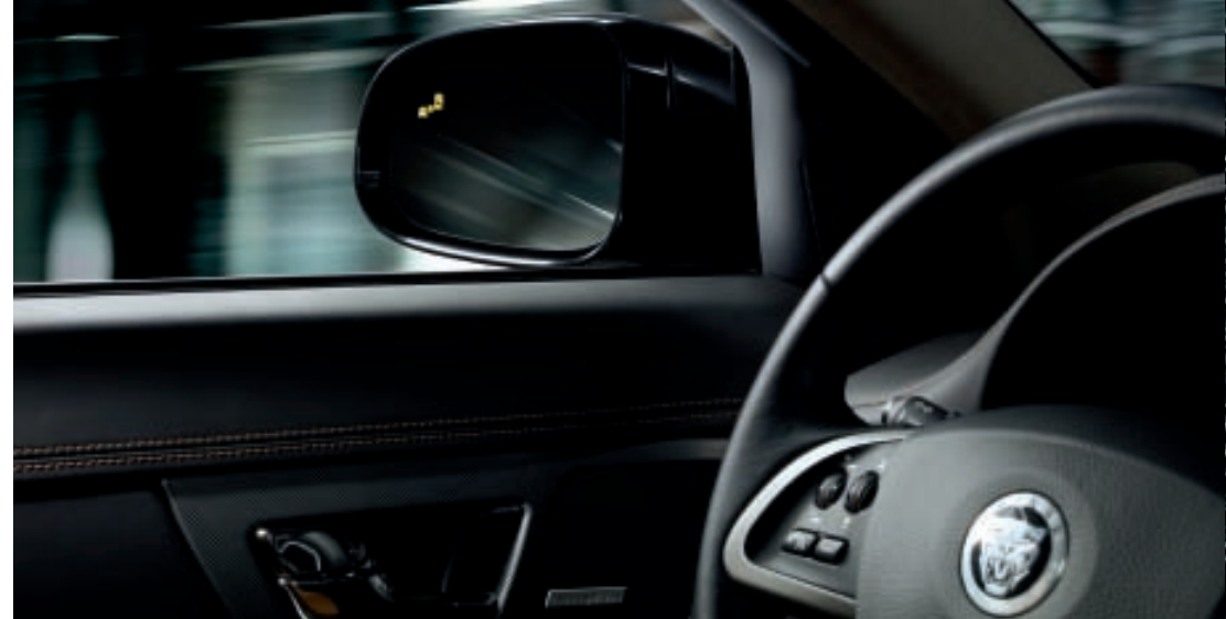
BLIND SPOT MONITOR* The Blind Spot Monitor uses side-mounted radar sensors to identify overtaking traffic and vehicles that cannot be seen in door mirrors or may be obscured. A bright amber warning icon illuminates in the appropriate door mirror when a hazard is detected to increase safety and driver awareness when changing lanes.
