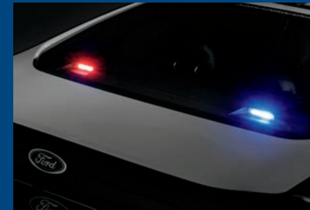
Police back-window lights. Includes (2) backlit flashing, linear high-intensity LED lights (driver side red; passenger side blue) mounted inside the decklid. Also with (2) backlit flashing, linear high-intensity LED lights mounted inside the decklid; lights activate when trunk is open.
