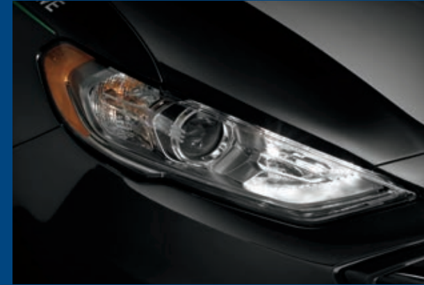
Police headlamp. Includes wide angle high-intensity LED lights (driver side red; passenger side blue).
