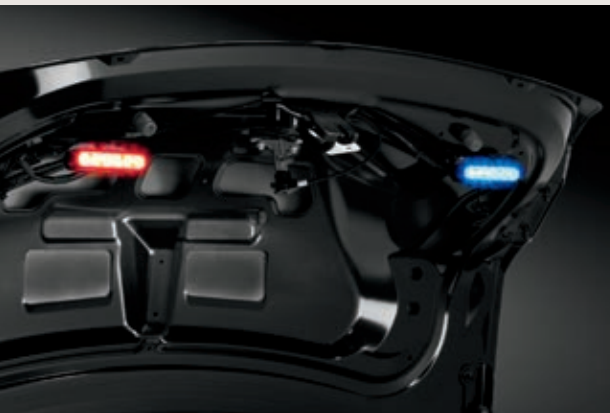
Police back-window lights. Includes (2) backlit flashing, linear high-intensity LED lights (driver side red; passenger side blue) with surround cover mounted inside the back window glass. Police trunk lights. Includes (2) backlit flashing, linear high-intensity LED lights (driver side red; passenger side blue) mounted inside the decklid; lights activate when trunk is open.
