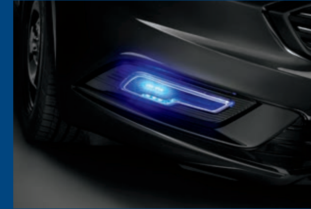
Front warning auxiliary lamps. Features integrated, custom-designed LED prep assembly.
