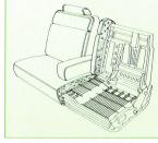
The Flight Bench Seat design helps promote driver-comfort. Molded-foam back padding is mounted directly to the steel seatback. And, a molded-foam seat cushion combines with a trampoline-like "Flex-O-Lator" steel mat to provide firm seat and thigh support.
