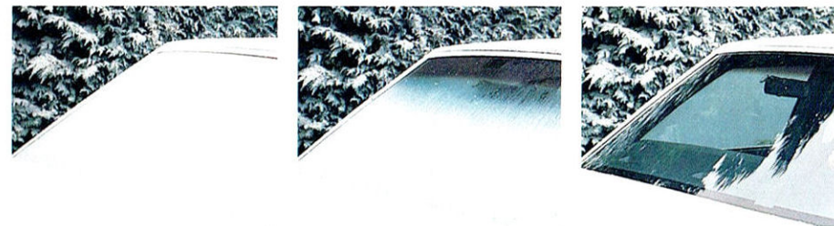
The Insta-Clear® heated windshield is an appreciated convenience in northern climates. It's capable of removing 1/10 of an inch of frost at 0 degrees Fahrenheit in just two to three minutes.
