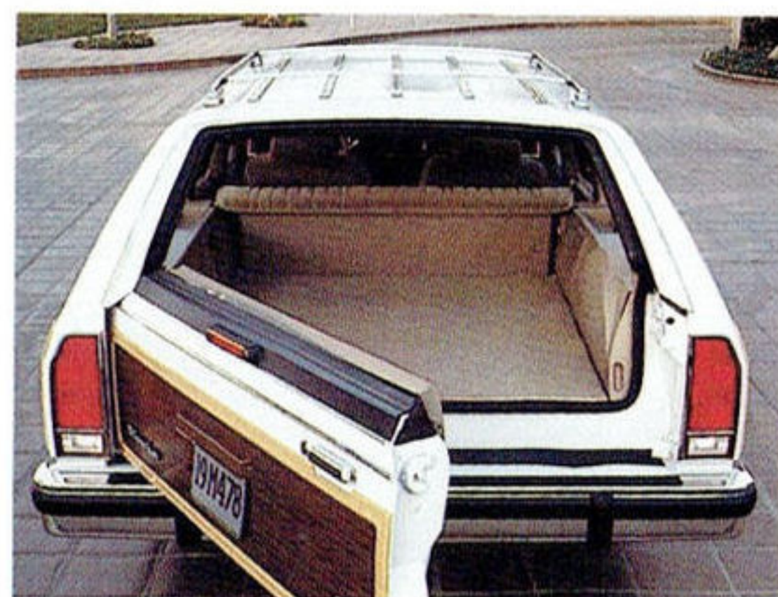
The 3-way doorgate on the wagon models opens to a spacious 88.2-cubic-foot cargo area.
