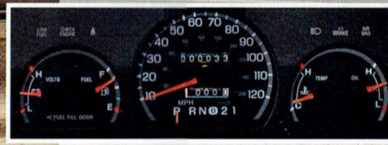
▲ The analog cluster includes gauges for battery charge, fuel, temperature and oil pressure.
