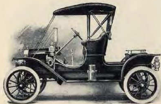
Model T Tourabout or Roadster, with rear seat removed and flat deck and rail ($9.00) substituted.
