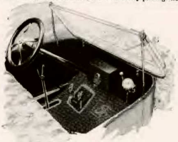
Showing the simplicity of the left hand control used on Ford Model T Cars
