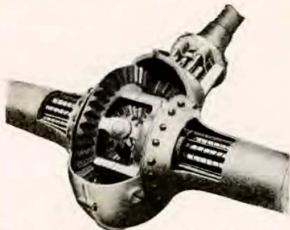
Three pinion bevel type Model T Differential, noted the world over for its simplicity and smooth running
