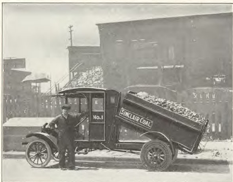
Truck with Dump Body, owned by J. C. Sinclair Coal Co., Detroit
