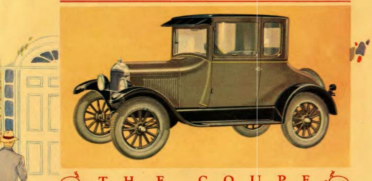
The Coupe is an exceptionally good looking car for personal use and the option of three attractive colors lends individuality. The body, with graceful pillars and excellent molding treatment, is of rigid all-steel construction. Standard equipment includes hooded sun visor, windshield wiper, rear view DETROIT mirror, dash light, nickeled radiator shell, starter and four balloon tires.
