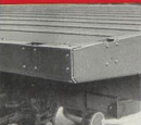
Platform rear corner showing steel frame rails, flush-set stake sockets and steel skid strips.
