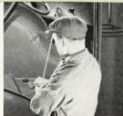
Hinged cover over handhole at bottom of engine cover provides quick access to engine oil level gauge.
