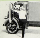
Wide doors, hinged at front, and convenient handholds provide easy access to cab for driver and helper.
