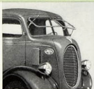
Excellent ventilation. Each half of divided windshield opens separately. Two large ventilators in cowl sides.
