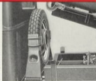
Channel side of dump truck spare wheel carrier is hinged so wheel can be rolled off.
