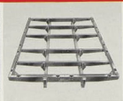
Bridge-type frame for platform body. Steel cross girders are riveted to steel frame rails.
