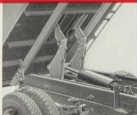
Optional arm-lift changes leverage ratio according to effort required to hoist body.
