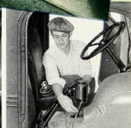
Convenient oil filler cap is on outside of engine cover. Tight-fitting rubber seal keeps fumes out of cab.
