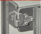
Stake rack sections are held tightly together at the top by bolted-on interlocking plates.
