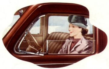
Controlled Ventilation is another new Lincoln-Zephyr feature. Tilting wings, operating independently of the front window, provide easily controlled ventilation. A large cowl ventilator is a welcome aid to comfort in warm weather.
