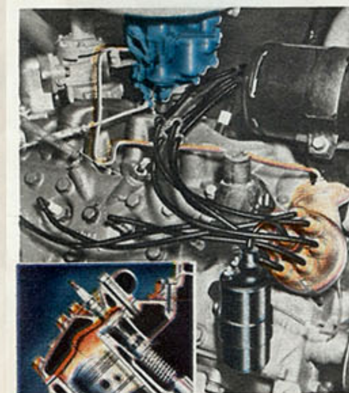
Automatic Mileage Maker . . . matches timing to fuel charges so every drop of gasoline is used—none wasted. Waterproof Ignition System, including snug synthetic rubber spark plug boots, prevents engine being shorted out by moisture.
