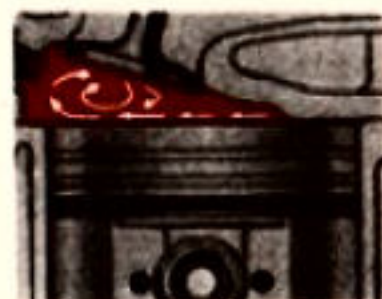
High-turbulence combustion chambers mix fuel and air thoroughly, burn fuel quickly, evenly and completely.
