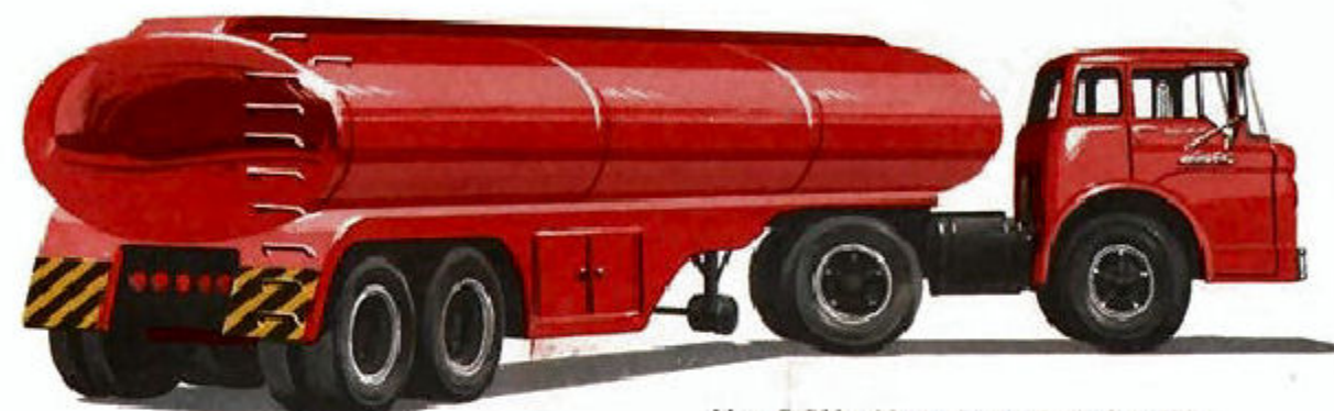
New C-800 with tandem axle tank trailer. Tractor wheelbases, 99 or 111 inches.
