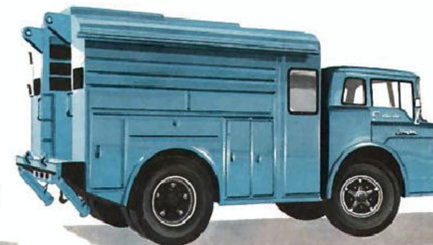
C-700 with Custom Cab and 13-foot line construction body on 135-inch wheelbase.
