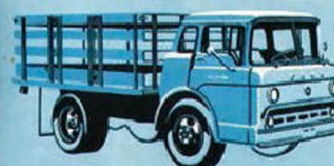
Husky 12-foot Platform-Stake body, factory installed on C-550. Nominal payload up to 11,310 pounds.
