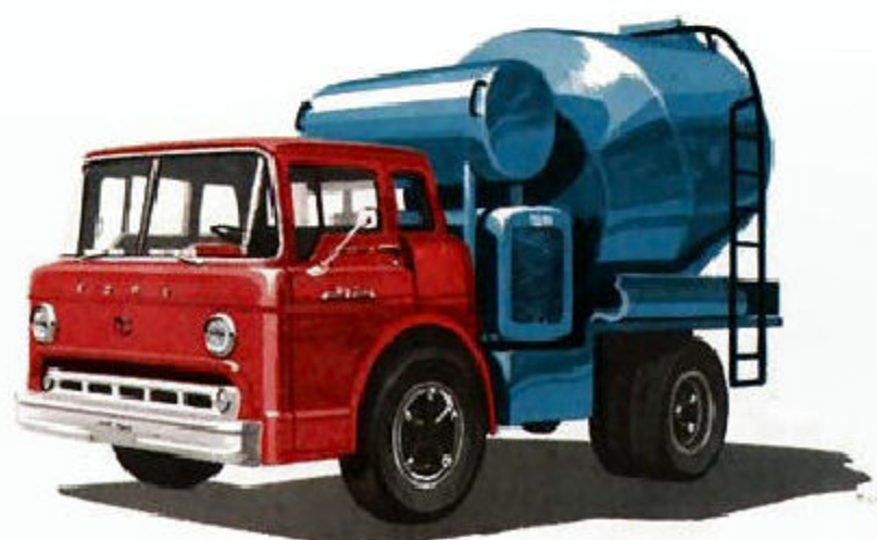
Concrete transit mixer on 111-inch wheelbase C-900. Compact and highly maneuverable with big load capacity. 212-hp HD V-8 with 4-barrel carburetor.
