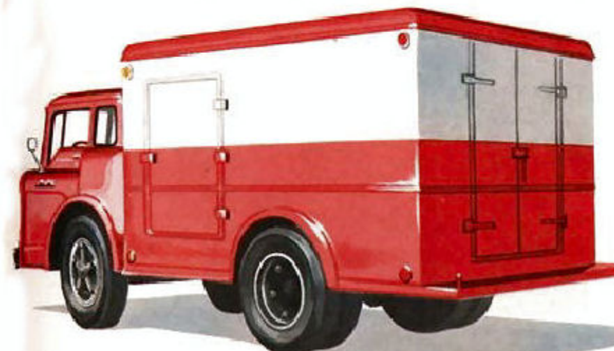
Ford C-700 with 12-foot refrigerated meat body, 111-inch wheelbase.
