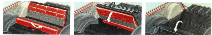
STOW-AWAY THIRD SEAT: Now, a forward-facing third seat that folds down into the floor. To store, simply pull seat release, push seat into seat well, fold down back. To open, release top, snap back, pull seat forward. When seat is in use there is a locking storage compartment beneath it.
