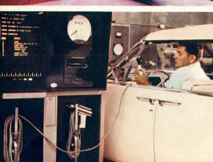
Every electrical circuit in each Lincoln Continental for 1962 will be individually checked by this electronic tester—which is so accurate that it not only detects failures actually present, but also makes sure each component draws just the right amount of current.
