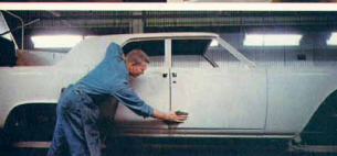
It takes more time, but careful hand-sanding of each coat of primer before the final color coat is applied, and meticulous attention to detail provide the kind of perfection in exterior finish the classic Lincoln Continental for 1962 demands.
