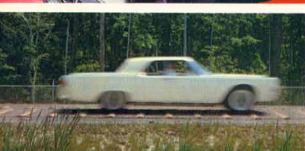
Culmination of Lincoln Continental's quality program is a 12-mile road test which every car goes through before leaving the factory. Specially trained driver-mechanics drive each one on a test track and on the highway.
