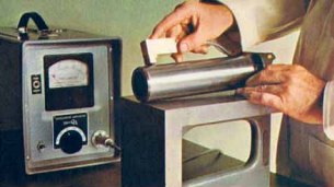
Special gauges and test equipment had to be developed to meet the exacting quality standards set for Lincoln Continental. Typical is this instrument which checks parts to millionths of an inch.
