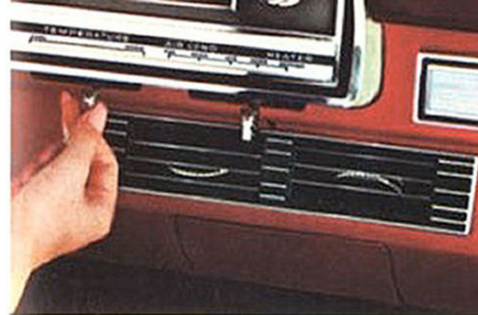
SELECTAIRE CONDITIONER: Air-conditioning, heating, defrosting are conveniently operated through a single control. Reheat feature removes moisture while cooling air.
