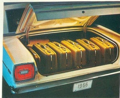
LOADS OF TRUNK SPACE. Ford trunk handles four 2-suiters upright with room on either side for more. Over 19 cu. ft. of usable space in all. Low sill, only slightly higher than the rear bumper, makes loading and unloading easier. Optional remote deck lid release unlocks trunk from the driver's seat.
