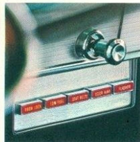
SAFETY/CONVENIENCE CONTROL PANEL. Includes (left to right): automatic door lock control, warning lights for "low fuel," "seat belts," "door ajar," control and indicator light for emergency flasher (simultaneous flashing of parking and taillights).
