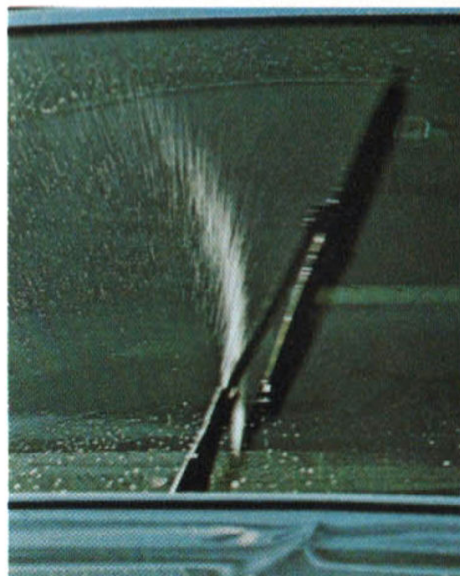
Wiper mounted windshield washer jet
