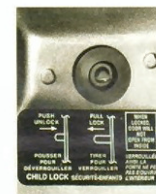
CHILD-PROOF SLIDING DOOR LOCK Setting this lock is accomplished simply by pulling out a button in the leading edge of the sliding
