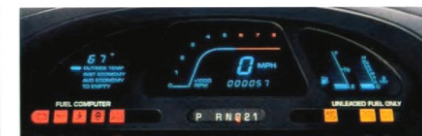
OPTIONAL ELECTRONIC INSTRUMENTATION Electronic instrument panel, available in Villager LS, provides digital speedometer and odometer readouts plus electronic graphics displays for tachometer, fuel level and engine temperature.
