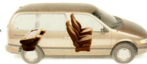
Three-passenger bench seat folded down and slid into third-row seating position one or two.
