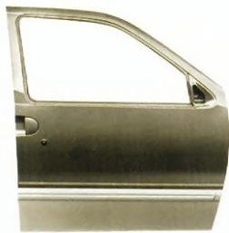
GALVANIZED BODY PANELS Protecting Villager from the elements begins with body panels of two-sided galvanized steel. Then an
