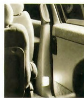
TIME-DELAY STEP LIGHT The step light remains on for 15 seconds after the ignition has been turned off, allowing time for rear seat
