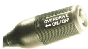
OVERDRIVE LOCKOUT SWITCH Gear selector lever contains a button which permits you to lock out the fourth-speed overdrive transmission function, providing increased engine braking when driving in hilly areas.
