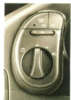
HANDY CONTROLS TO YOUR LEFT Conveniently grouped controls at the left of the steering wheel turn headlamps on/off, adjust instrument panel brightness and, in LS models, activate speed control and available autolamp delay systems.
