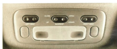
OVERHEAD CONTROLS In Villager LS, the optional power moonroof is controlled from an overhead console which also contains controls for map lights and power rear quarter windows.
