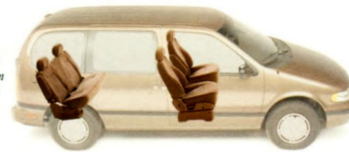
Three-passenger bench seat in third-row seating position one. (It slides back farther for seating position two.)
