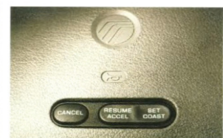
FINGERTIP SPEED CONTROL After activating the speed control with the instrument panel switch, you set the desired speed with these buttons. Note their convenient location near the center of the steering wheel, close to your hands.
