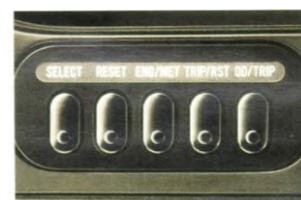
FUEL COMPUTER Included in the available LS electronic instrument panel, it permits you to call up readouts for instant fuel economy, average fuel economy and distance to empty. Other functions are outside temperature and trip distance.
