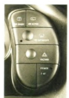
AND TO YOUR RIGHT Cluster at the right of the steering wheel contains controls for rear washer/wiper and defogger. Also located here are switches for hazard flashers and the Power E-AT function which is described in text on this page.
