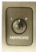
OUTSIDE REARVIEW MIRROR CONTROL Dual power outside mirrors are standard on LS, optional on GS.
