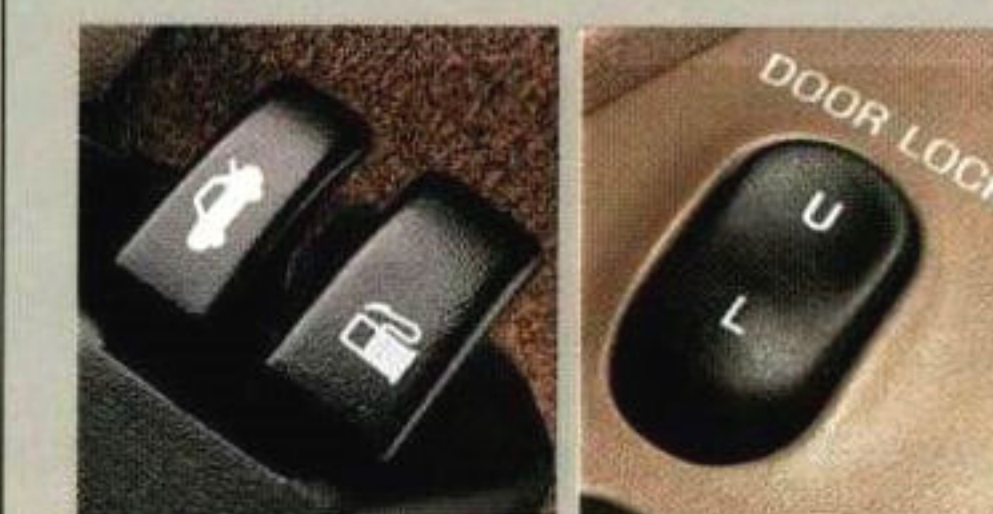
POWER LOCK GROUP. Includes power door locks, decklid release and fuel-filler door release.
