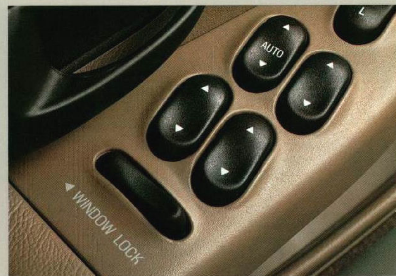
POWER WINDOWS. Operated by illuminated controls. Includes driver override feature.
