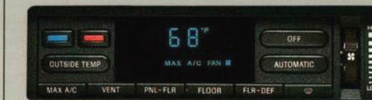
ELECTRONIC AUTOMATIC CLIMATE CONTROL. CFC-free system automatically maintains the temperature you find most comfortable.
