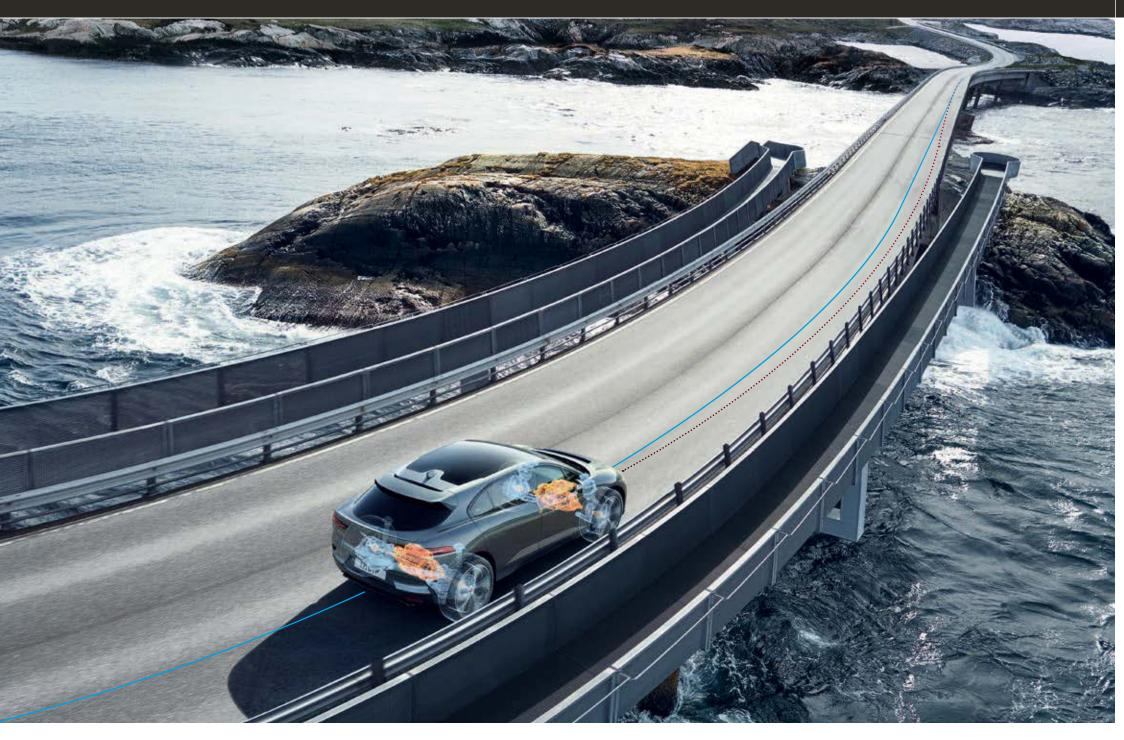
Torque Vectoring by Braking applies brake pressure to slow the inside front or inside rear wheels independently helping to prevent understeer and stay on the true line of travel
