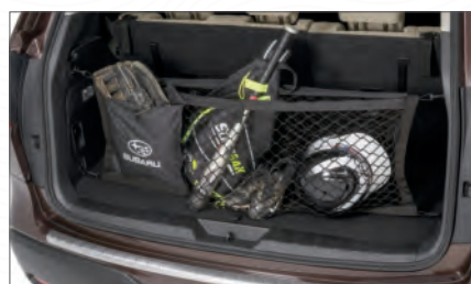
Cargo Net. Neatly holds cargo and prevents it from sliding while the vehicle is in motion. The Cargo Net can be used two ways: anchor it to the sides of the cargo area to help prevent shifting from front to back or lay it across the floor to help keep things from rolling around.
